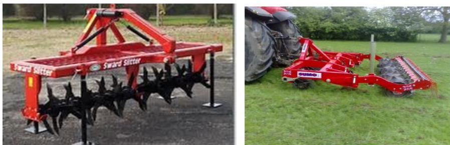
Typical equipment for spiking or sward lifting to alleviate shallow compaction.
